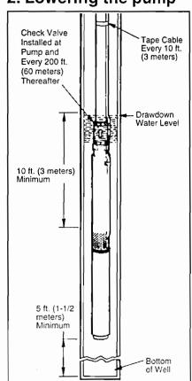
a) Align pump carefully when beginning to lower it down the well casing. Do not let the pump, cables or pipe rub against the well casing. Take care that cable insulation is not dragged or scraped over the top lip of the well casing.
